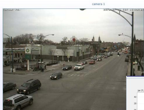
Observation @ 26.01.2010 16:20 Air Temp 21.9 °F **Dew Point Temp** 12.7 °F Rel Humidity 67 % Surf Temp 30.9 °F Surf State none Grip Level 0.82 Water Layer 0.0 in Ice Layer 0.0 in Snow Layer 0.0 in Can compare air temperature and surface temperature in real time
