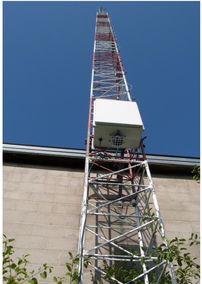
*Wet Bulb Globe Temperature Sensor*
