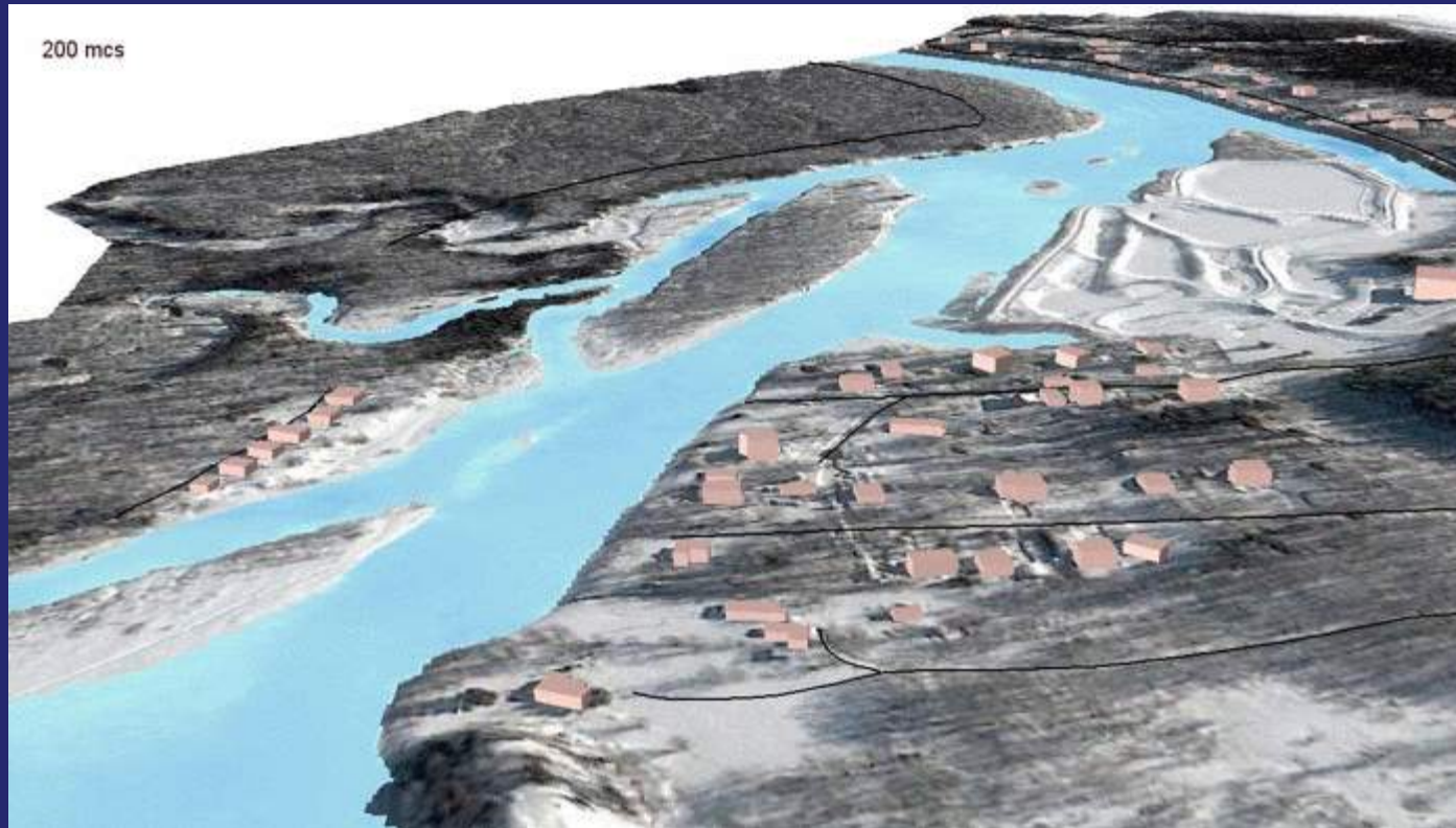
Simulation of flooded areas for different flows, Montmorency River, Quebec
